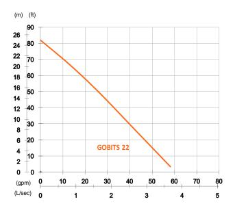
Shaft Speed: 3450 rpm Outlet: 50mm, 2in
